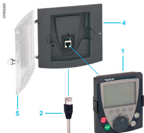
Using the graphic terminal on enclosure door: 1 + 2 + 4 (+ 5, if IP 65)
